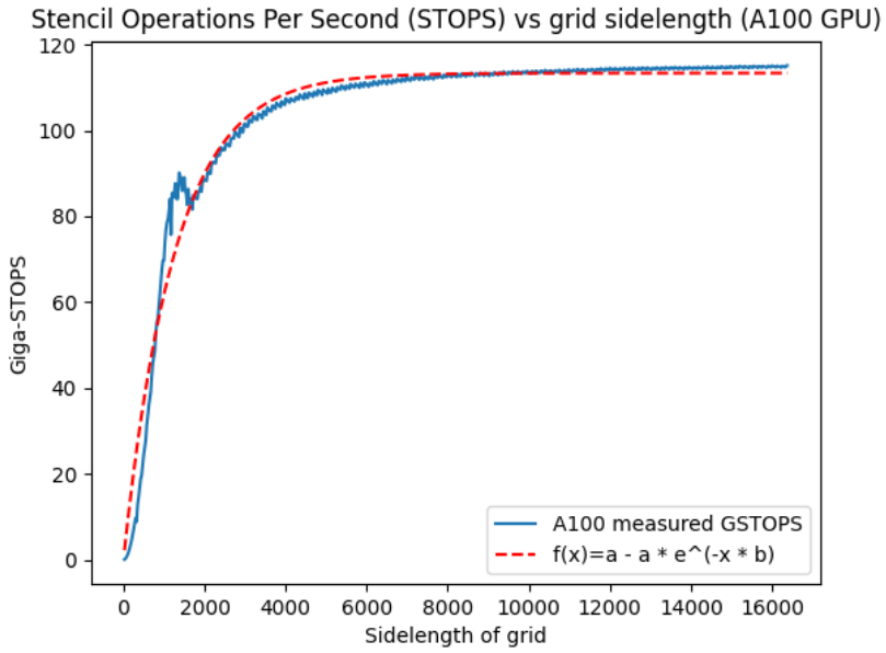
Figure 7.19: GSTOPS vs. grid size for the A100 GPU
