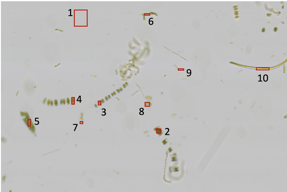
Figure 9.18: RGB representation of the hyperspectral datacube using wavelengths R=630 nm, G=550 nm and B=480 nm, with bandpass of 5 nm. (1) background area, (2, 3, 4, 8) diatom Thalassiosira , (6, 7, 9) diatom Chaetoceros and (10) diatom Fragilariopsis .
