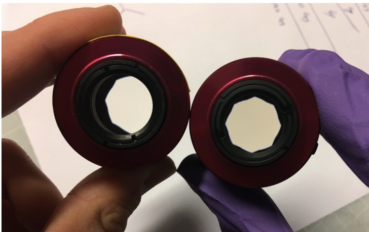
Figure 6.11: Non-irradiated objective (to the left), next to the irradiated objective (to the right). The irradiated objective is visually more brown in color.
