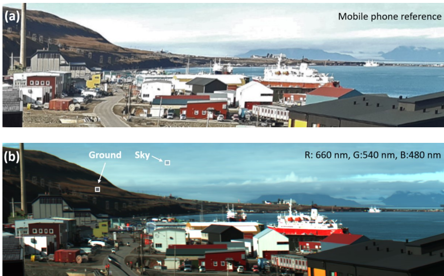
Figure 3.9: Longyearbyen harbor, 26-08-2019. (a) Mobile phone image, for reference. (b) RGB image generated from the hyperspectral datacube, using wavelengths 660 nm, 540 nm and 480 nm. Data from [139].
