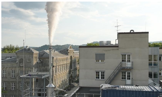
Figure 2: Image of CO 2 plume released from the exhaust pipe in depressurization test 4.
