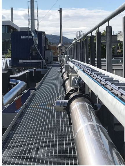
Figure 6.2: The ECCSEL depressurization tube. The CO 2 is vented through the stack in the background. Photo taken by Han Deng at SINTEF Energy Research.
