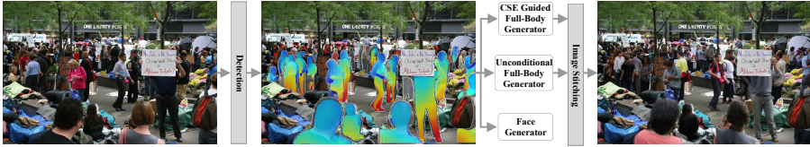
Figure 3.5: DeepPrivacy2 supports multi-modal anonymization, where three detection and synthesis networks are employed: (1) a CSE-guided generator for individuals detected with dense pose (by CSE (Neverova et al. , 2020)), (2) an unconditional full-body generator for cases where CSE fails to detect (note the segmented persons without color-coded CSE detections), and (3) a face generator for the remaining individuals (marked in red). The original image is from Wider-Face (Yang et al. , 2016).
