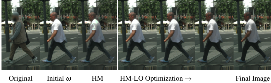
Figure 4.1: The global context mismatch problem refers to the issue where the synthesized identity may not align with the global context of the image, making the synthesized identity "stick out". Note that the illumination of the synthesized identity ("initial \omega ") is different from the original identity. Paper F explore two options to address this issue: naive histogram matching ( HM ), and histogram matching via latent optimization ( HM-LO ), which iteratively adjusts the initial \omega to better fit the histogram of the original image (in HSV). See Paper F for further details.
