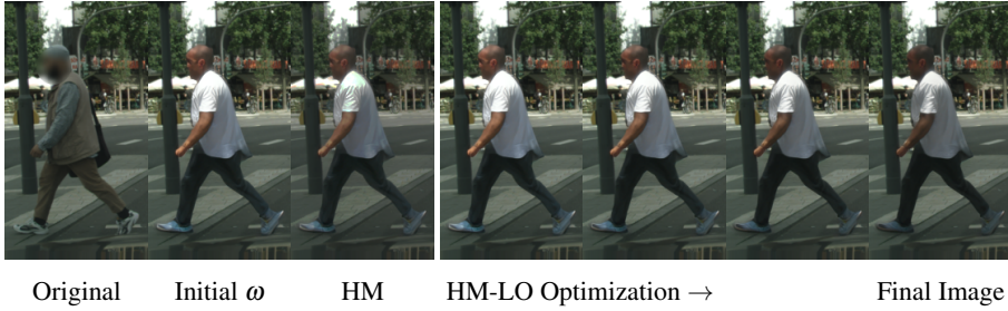
Figure 4: The initial synthesized identity ("initial \omega ") may not align with the global context of the image, making the synthesized identity "stick out" compared to the original identity. We explore two options to address this issue: naive histogram matching ( HM ), and Histogram matching via latent optimization ( HM-LO ), which iteratively adjusts the initial \omega to better fit the histogram of the original image (in HSV)
