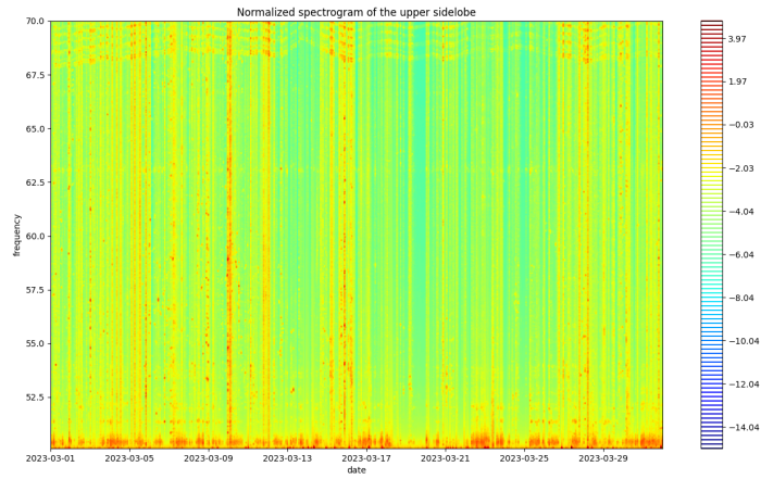
Figure A.10: The upper sidelobe in March normalized on the 50 Hz signal magnitude. Here the modulated signals are more clearly visible. We can however still see a clear influence of the varying intensity of the 50 Hz signal.
