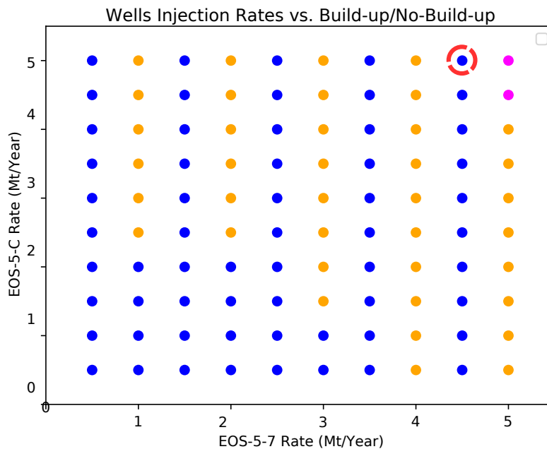
Figure 6.1: Well injection rate balance 2D plot for the BHP limit of 400 bar.
