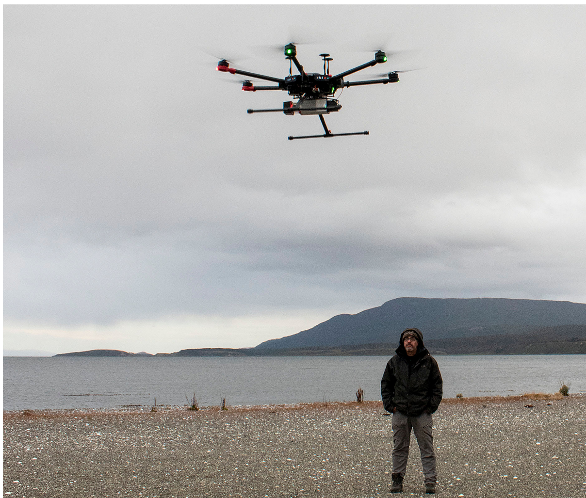
FIGURE 11 We used a Riegl miniVUX-3 UAV LiDAR sensor mounted on a DJI Matrice 600 Pro drone, here in action in Tierra del Fuego. Photo: Ole Risbøl. [Colour figure can be viewed at wileyonlinelibrary.com ]
