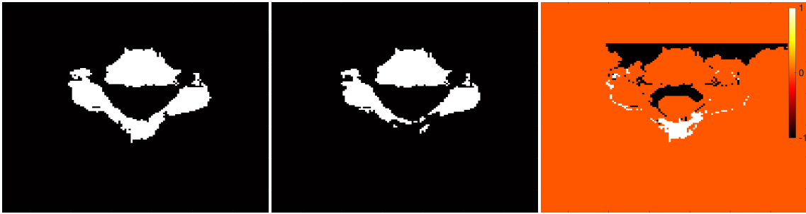
Figure 29: Visualisation of how the automatic segmentation method performs compared to the manual segmentation for the fifth subject. From left to right, a) the manual segmentation, b) matrix containing similarities, "true positives", and c) the difference, "false positives" in black and "false negatives" in white
