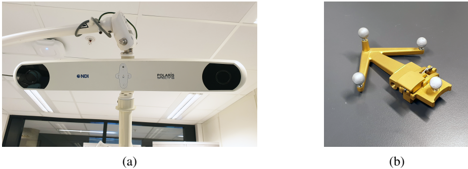
Figure 3.2: (a) NDI POLARIS Spectra® (NDI, Toronto, Canada) and (b) a marker shield with a gripper for ultrasound (US) probes and passive reflective markers.
