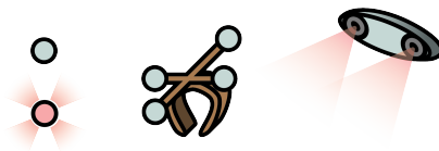
Figure 3.1: Optical tracking system (OTS). From left to right and top to bottom: passive markers, active markers, frame or marker shield with passive markers and infrared cameras.
