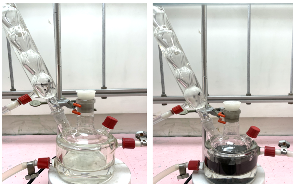
Figure 5.2: 1) Water leaching setup 2) Leaching setup with black mass.
