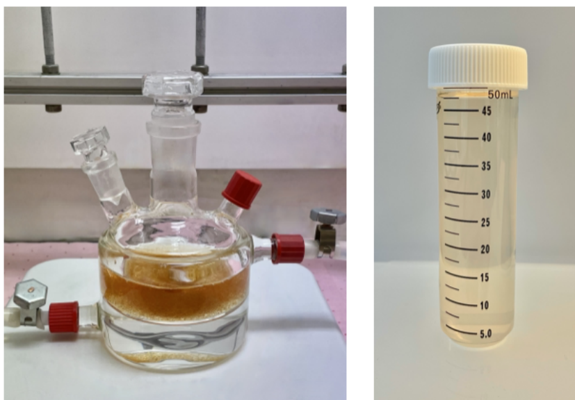
Figure 5.5: 1) Batch reactor setup for adsorption experiments. 2) Li-depleted solution after filtration.
