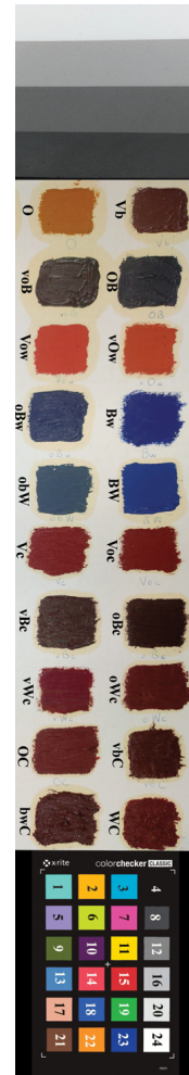
Figure 3. Acquisition arrangement of pigment mockup with the Spectralon ® multi-step reference target to the left and ColorChecker on the right. Numbering for ColorChecker is added manually here in this figure for reference.
