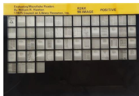
Figure 1. An example of a positive microfiche, of physical dimension 105mm × 148mm and a reduction ratio of 24X or 24 times, which will be used in the assessment of text legibility experiment. This material comes from Ref. [14].
