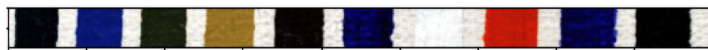
Figure 4. A snippet of a mockup with ten pigments and substrate; Colors are approximated as RGB rendering using spectral python for bands 75, 46, and 19 of HSI datasets.
