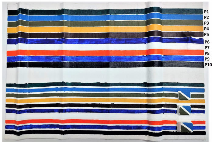
Figure 2.1: Pigment mockup B; mockup was prepared using pigment tubes composed of high-stability pigments and oil, purchased from Zecchi (ZECCHI 2023). The pigments were selected based on three main factors: their prominence in CH research articles, their specific spectral characteristics, and consultation with experts in the CH field. Veridian(P1), Cerulean Blue(P2), Green Earth(P3), Yellow Ochre Light(P4), Burnt Umber(P5), Ultramarine Blue Deep(P6), Lead White Hue (P7), Genuine Vermilion(P8), Cobalt Blue Deep(P9), and Ivory Black(P10) are pigments used in the mockup. The linen canvas was primed using three layers of white gesso before applying these pigments.
