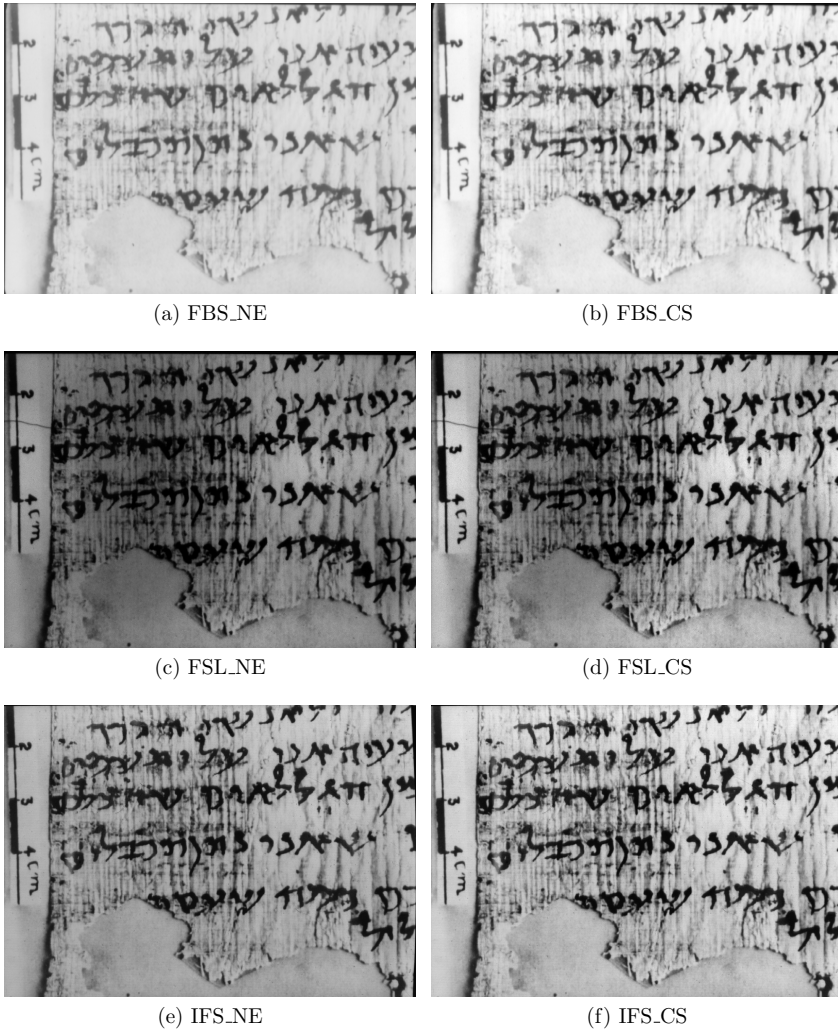
Figure S4: Microfiche images with fragments showing images with enhancement (.CS) and without enhancement (.NE). Image from flatbed scanner (FBS), microform reader (FSL), and in-house film scanner (IFS).
