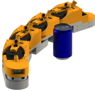
Figure 3.11: A digital render of a 5-link Boa snake robot, with a soda can for scale reference.
