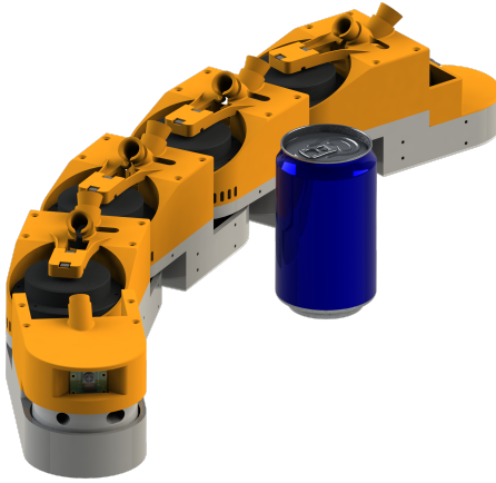
Figure 3.4: A digital render of a 5-link Boa snake robot, with a soda can for scale reference.
