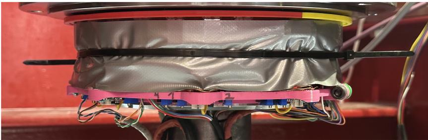
**Figure 3.9:** The amplifier assembly mounted on the turbine shaft and connected to the slip ring (out of frame)
