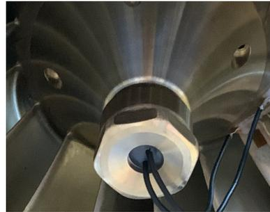
(b) Closeup of the cone during assembly. *Note that the wires were yet to be tucked close to the cone surface and tied down at this point.*
