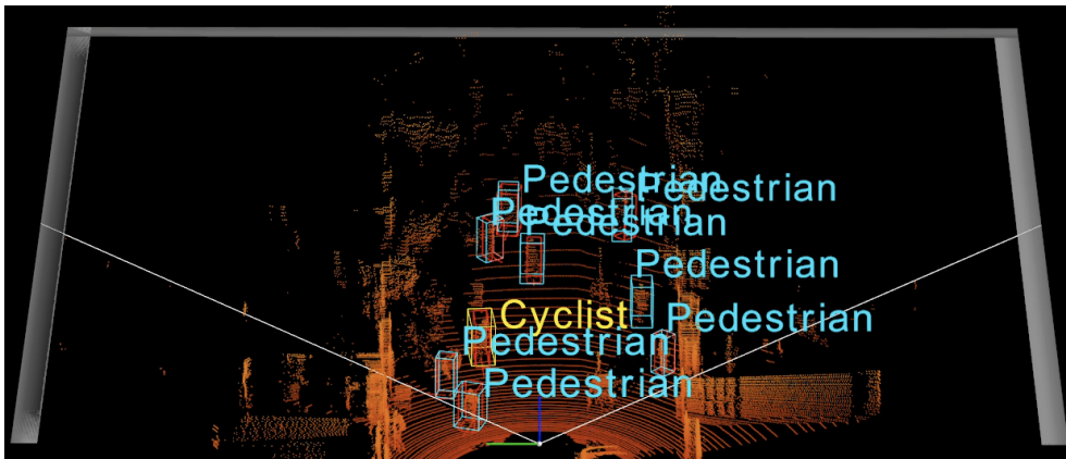
Figure 4.20: Far velodyne-visualization of point cloud with blue and yellow boxes as ground truth and red boxes as the model predictions. Red lines indicate orientation
