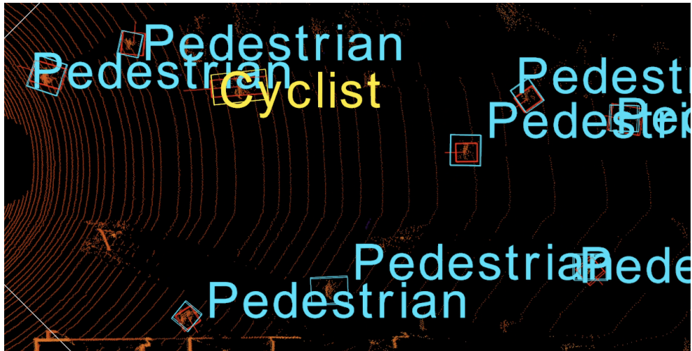
Figure 4.23: BEV-visualization of point cloud with blue and yellow boxes as ground truth and red boxes as the model predictions. Red lines indicate orientation
