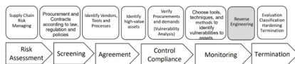
Figure 2: Proposed inclusion of a Reverse Engineering subprocess into the equipment procurement process at a DSO
