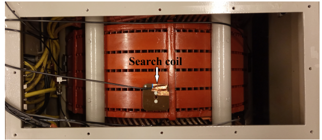
Fig. 10. The location of non-invasive search coil sensor to capture the stray magnetic field installed on the back-side of the stator yoke.
