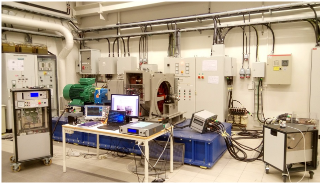
Fig. 8. The experimental test rig of a 100 kVA synchronous generator with 14 salient poles.
