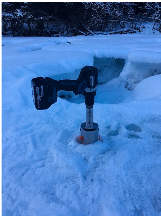
Fig. 6. Ice core extraction in process on anchor ice dam 1.
