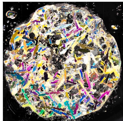
D – Frazil small needles (8 samples) Ice Dam 2, Core 5, 60 cm from top
