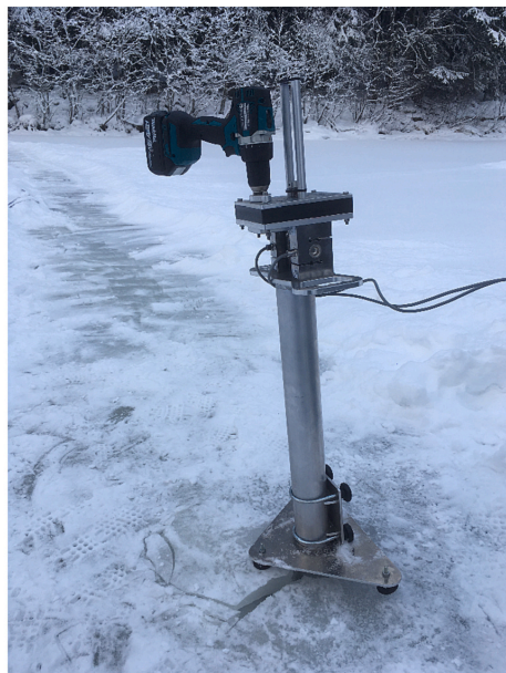
Fig. 8. Schematic of a borehole-jack (BJ) similar to the one used in this study (Kallelid, 2018).
