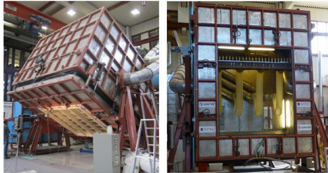
Fig. 1. Large-scale turnable box for rain and wind tightness testing of sloping building surfaces (RAWI box). Test running with a test sample (left) (Breivik et al., 2013), and RAWI box without a test sample (right) (Andenas, 2016).
