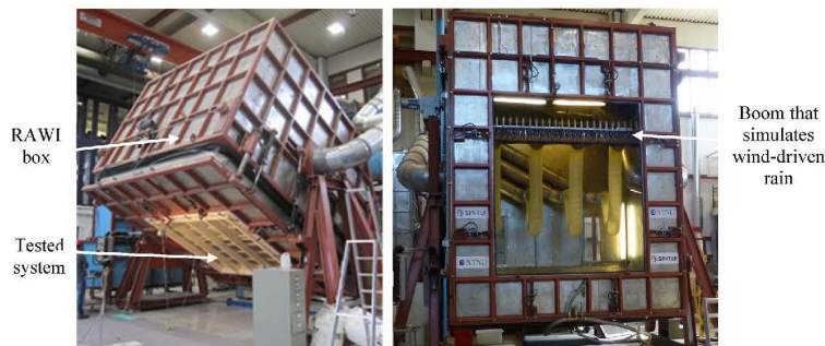
Fig. 1. Large-scale turnable box for rain and wind tightness testing of sloping building surfaces (RAWI box), while test is running (left) [20] and RAWI box without a test sample (right) [21]. Schematic drawing of RAWI box is shown in Fig. 12.
