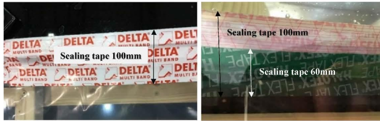
Fig. 6. View of a complete taping from the frontside (left) and from the backside (right). Study 3 (Table 3).
