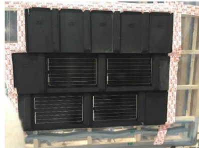
Fig. 8. Front view of the outline of BIPV roof tile system. To distinguish solar tiles from matching tiles they are coloured in dark grey and black (solar tiles) and light grey (matching tiles). As depicted on the picture on the right, in reality both types of tiles have the same black colour. Here BIPV roof tile system shown with completed taping before laboratory testing. Front view of the exterior BIPV system side.
