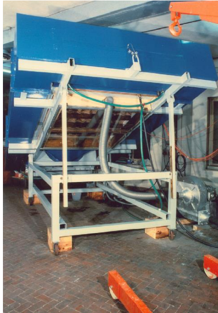
Figure 23. The apparatus used for waterproofing tests, the transparent box under the sample is visible [106].
