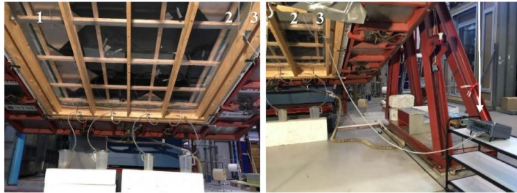
Fig. 13. Raintightness test setup in the laboratory. The set of 3 tubes to measure air pressure difference are marked. Tube 1 for measuring the differential air pressure by the RAWI box, and tubes 2 and 3 for measuring the differential air pressure connected to the external micromanometer. Study 3 (Table 3).
