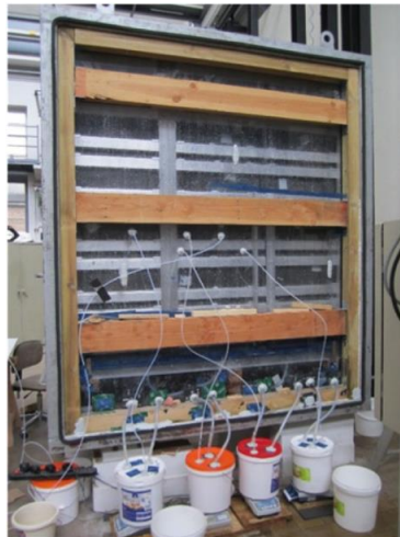
Figure 27. Photo of the laboratory setup of the rear face of the mock-up. The collection trays are connected with plastic tubes to buckets placed on weighing scales, which measure the water ingress [111].
