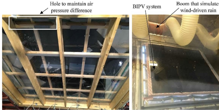
Fig. 10. The BIPV system during trial runs viewed from the outside (left) and inside (right) of the RAWI box. Study 3 (Table 3).
