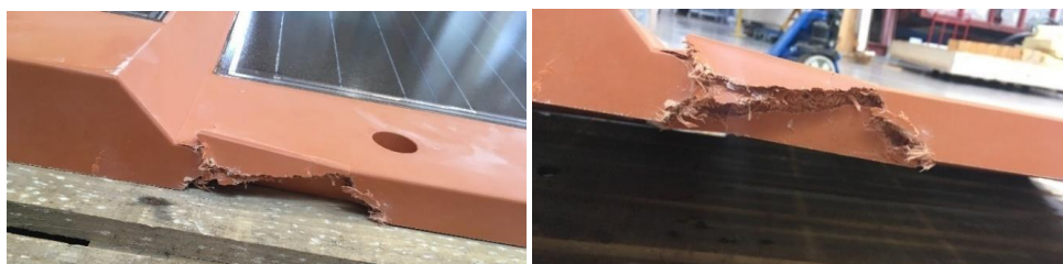
Figure 59. The fourth BIPV system that was received for testing but was not tested due to severely damaged during transportation.
