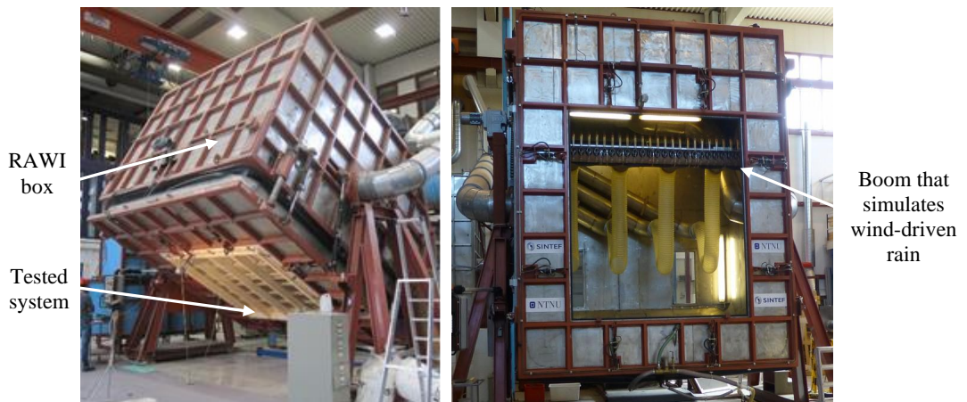
Figure 30. Large-scale turnable box for rain and wind tightness testing of sloping building surfaces (RAWI box), while test is running (left) and RAWI box without a test sample (right) [114]. Schematic drawing of RAWI box is shown in Figure 29.
