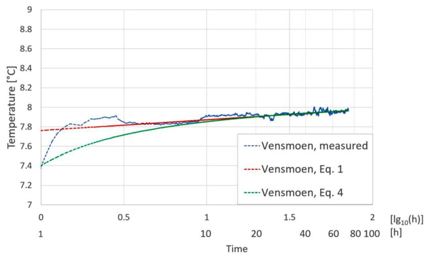
Fig. 5. Measured and modelled temperatures for the TRT results at Vensmoen: Time is given on a logarithmic scale with base number 10 and corresponding values in hours below.
