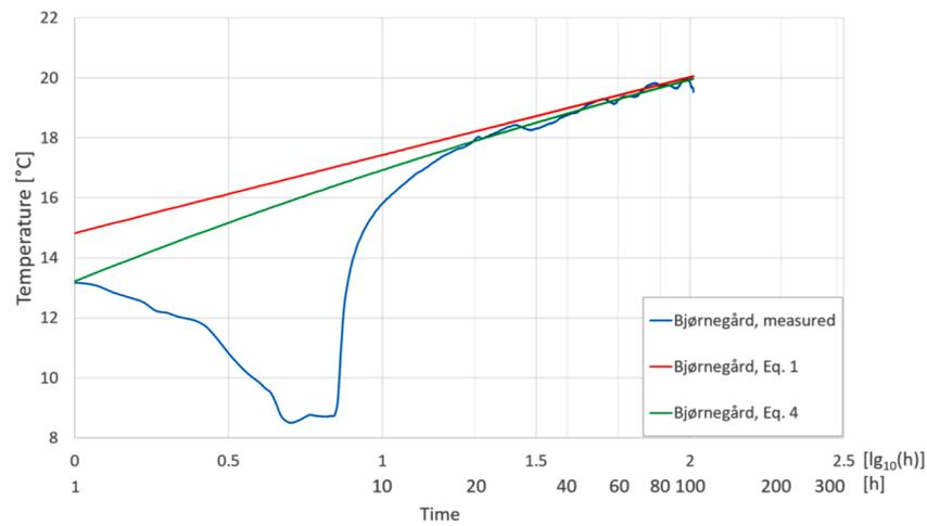
Fig. 3. Measured and modelled temperatures for the TRT results at Bjørnegård: Time is given on a logarithmic scale with base number 10 and corresponding values in hours below.
