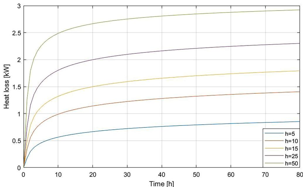
Fig. 7. Theoretical heat losses due to advection during TRTs where 40 W/m is injected, 100 m of the borehole length is affected by convection with a given advection coefficient  $h$  [W/(m<sup>2</sup>K)] and the borehole radius is 5.75 cm.  $h = 5$  W/(m<sup>2</sup>K) is close to the values for Lillås and Bjørnegård and  $h = 50$  is a very high value, similar to that at Vensmoen.
