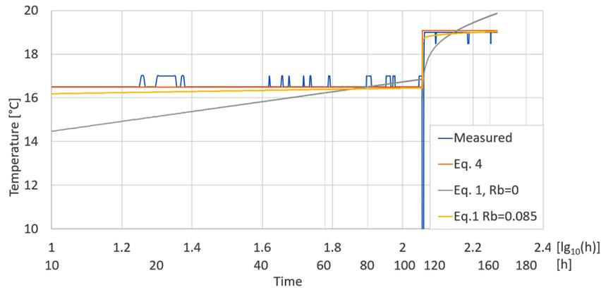
Fig. 6. Using Eq. (1) and (4) to fit the temperature data from Herford, Germany with  $R_b$  set to 0 or 0.085 W/(mK): Time is given on a logarithmic scale with base number 10 and corresponding values in hours below.
