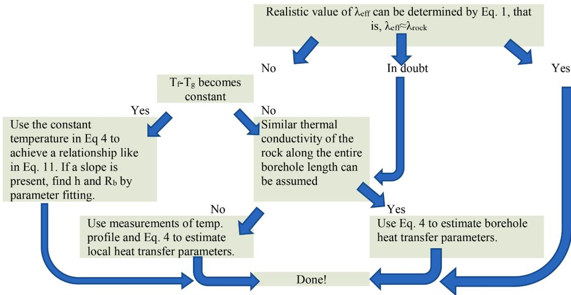
Fig. 9. Suggested procedure for when to use Eq. (1) and when to use Eq. (4).
