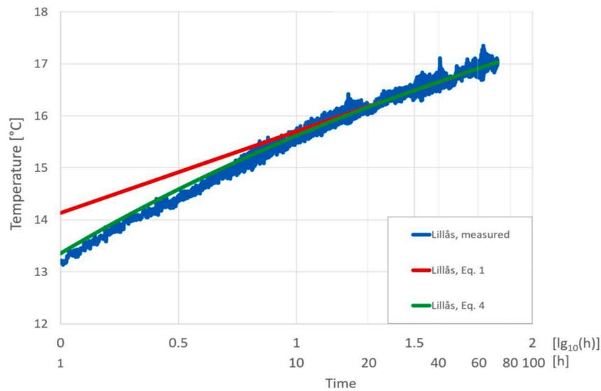
Fig. 4. Measured and modelled temperatures for the TRT results at Lillås: Time is given on a logarithmic scale with base number 10 and corresponding values in hours below.
