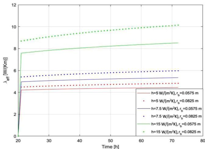
Fig. 8. Result of applying linear regression and Eq. (1) to temperature series developed with Eq. (4) with  $\lambda_{\text{rock}} = 2.9$  W/(mK).
