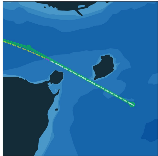
Fig. 3 A demonstrative path following simulation using MPC, not including any risk cost terms in the cost function
