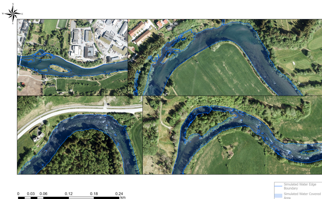
FIGURE 3 Comparison of simulated (blue transparent surface) with aerial imagery for the hydraulic simulation of Eidselva. Source: aerial imagery www.norgebilder.no , Courtesy: Statkart and the Geovekst project. [Color figure can be viewed at wileyonlinelibrary.com ]
