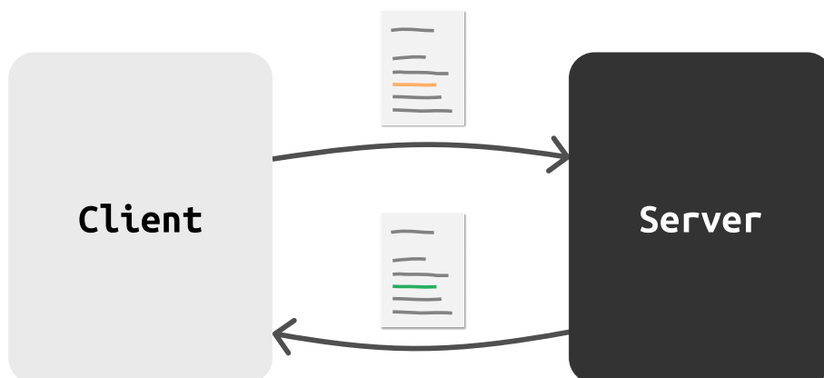
Figure 7.2: Overview of a mutation operation. The client initiates a mutation request, denoted by the orange line, indicating mutated data. The server, in response, potentially provides the modified version of the same data, represented by the green line.
