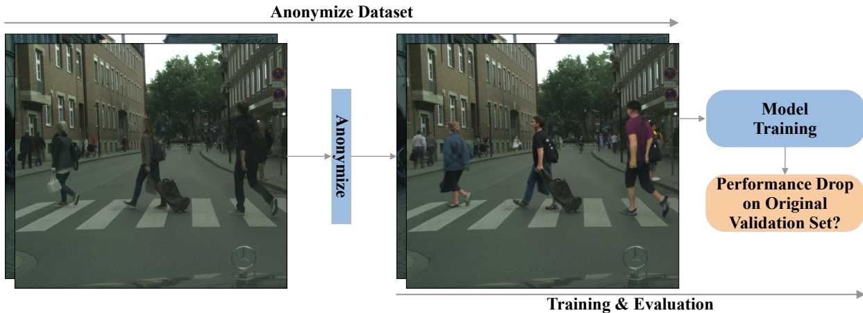
Figure 1. To assess the impact of anonymization, we first anonymize common computer vision datasets, then train various models using the anonymized data, and finally evaluate the models on the original validation datasets. The figure depicts our Cityscapes [8] full-body anonymization experiment. Note that the leftmost image is anonymized with face blurring, following Cityscapes [8] terms of use.
