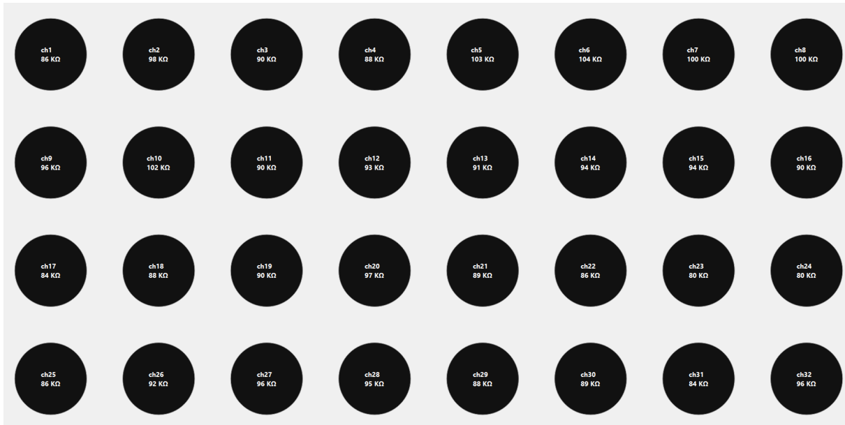
(b) Impedance on all channels for participant no. 6. This participant had the highest impedance after the set-up time of 30 min.
