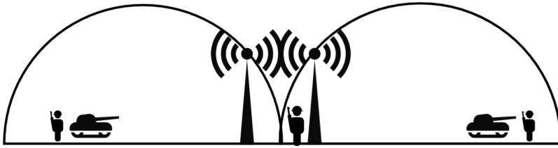
Figure 2.1: The relay station in the middle of the picture is connecting the two bubbles allowing them to communicate with each other
