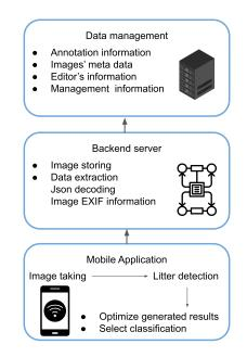
Fig. 1: Architecture for the proposed system for litter monitoring based on a mobile application.
