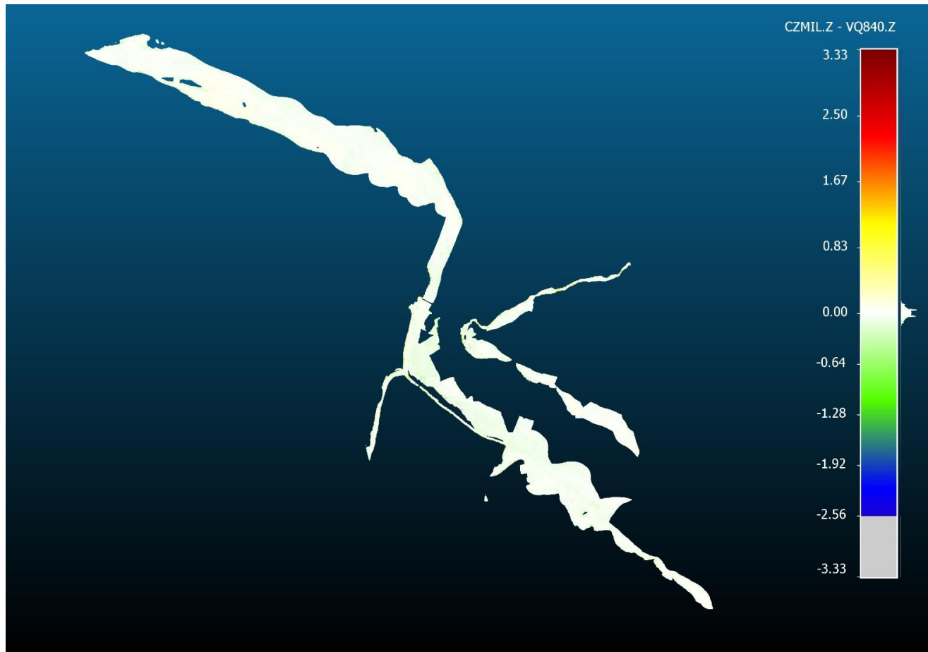
Figure 19. Residual map for the Green LiDAR bed elevations for CZMIL against Riegl VQ840 in Krøderen.
