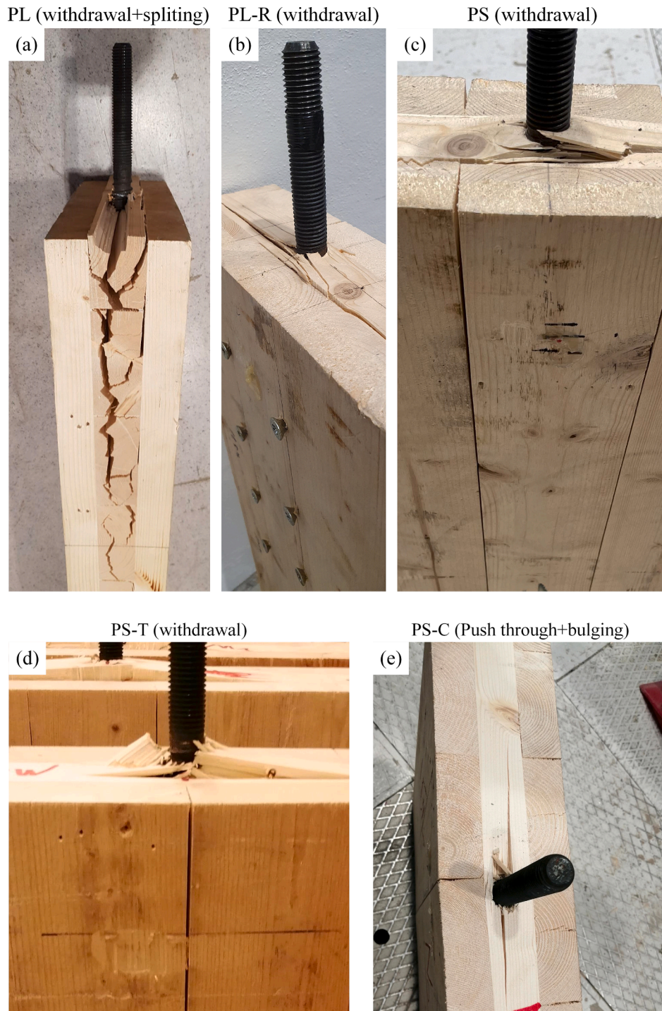
Fig. 15. Failure modes of all test series.
