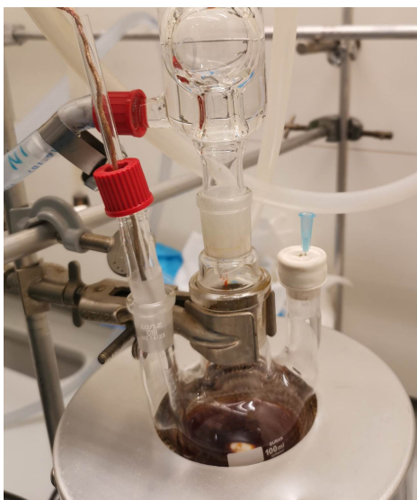
Figure 3.2: Photo of the thermal decomposition set-up for the IONP synthesis. The same set-up was used for NS and NC synthesis, consisting of a three-necked round-bottom flask, condenser, Ar gas, magnetic stirrer, and a temperature probe.
