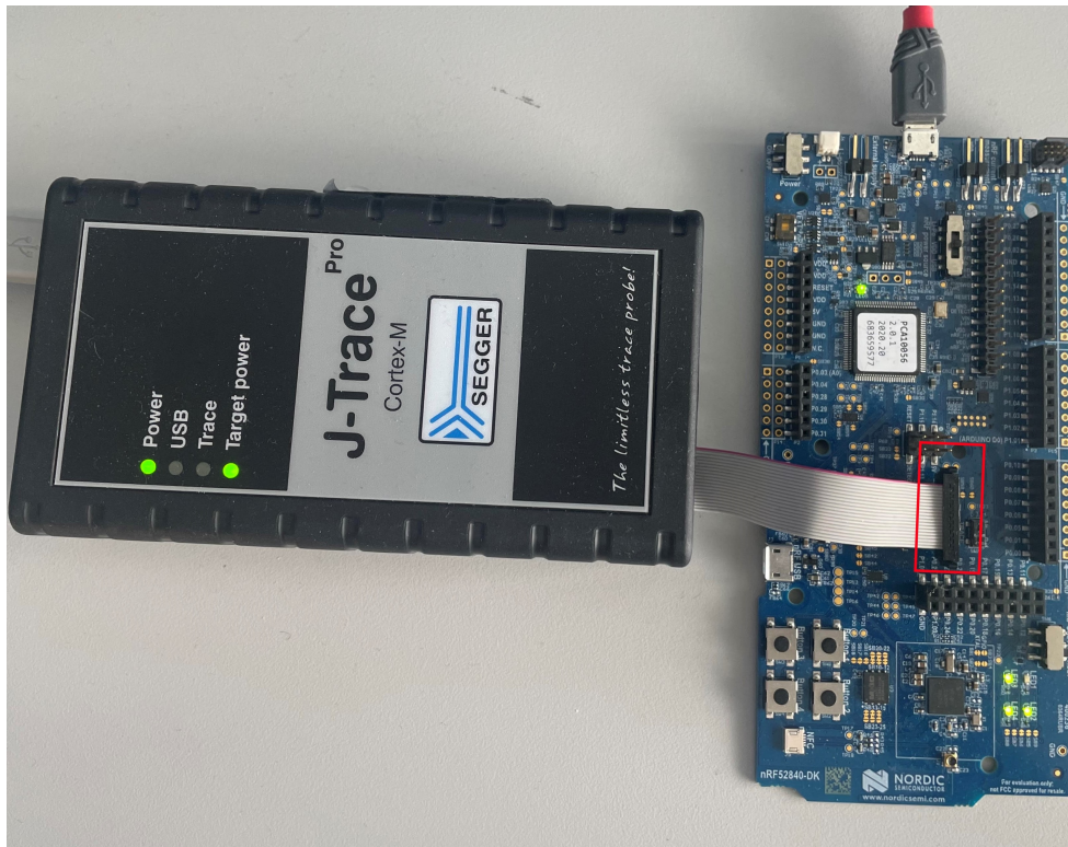
Figure 3.2: nRF52840 with the 20 Pin Interface Soldered.
