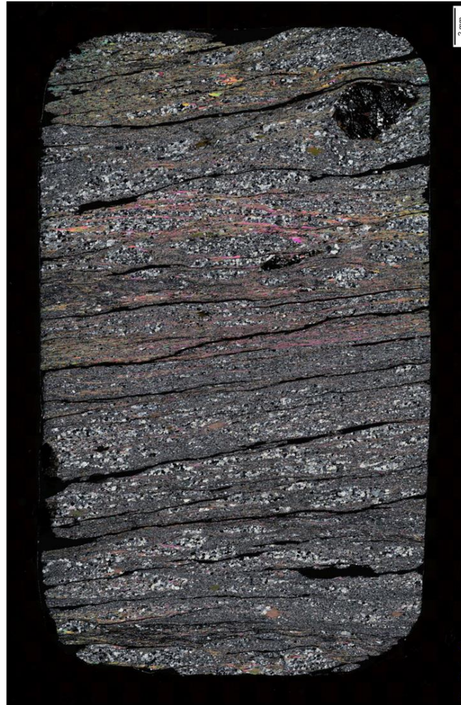
Thin section 2-2 displayed in PPL with the polarizer rotated by 90° and XPL at 45°. The whole thin section was analysed with SEM, creating an overview map and the red rectangles represents the area for the detailed maps.
