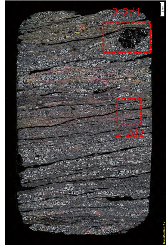
Thin section 2-2 displayed in PPL with the polarizer rotated by 90° and XPL at 45°. The whole thin section was analysed with SEM, creating an overview map and the red rectangles represents the area for the detailed maps.
