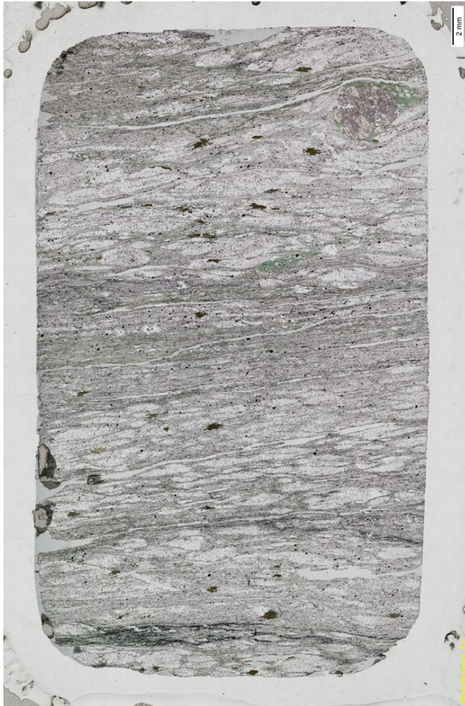
Thin section 2-2 displayed in PPL with the polarizer rotated by 90° and XPL at 45°. The whole thin section was analysed with SEM, creating an overview map and the red rectangles represents the area for the detailed maps.
