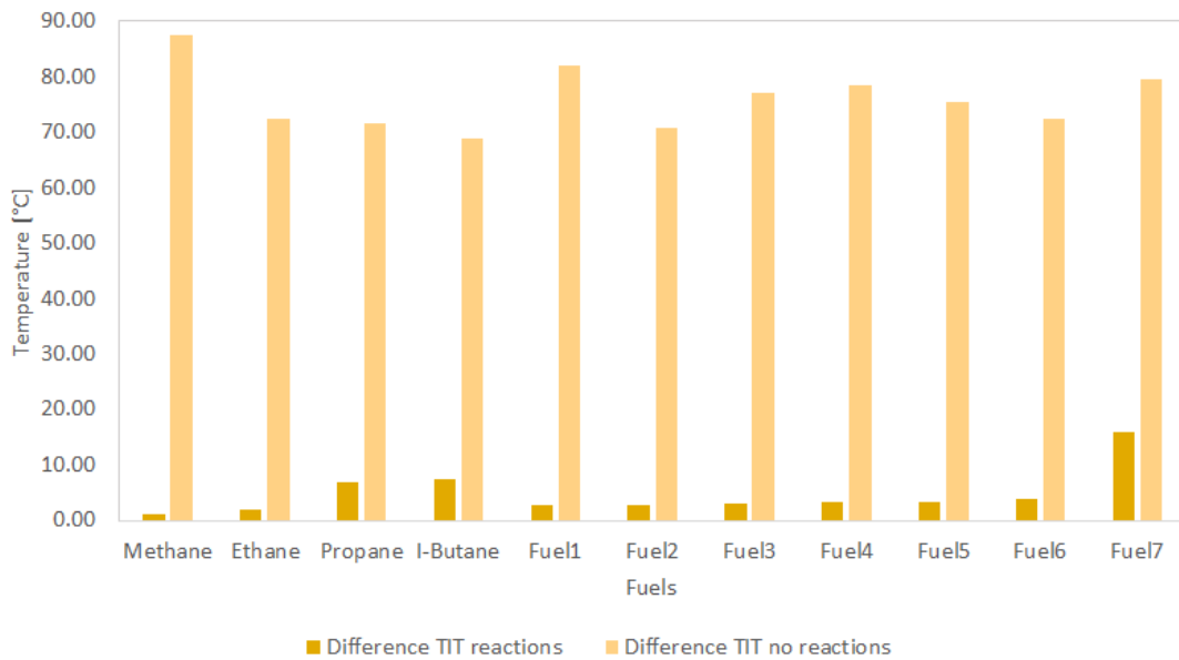
Figure 4.1.11: Comparison between the absolute difference of the TIT in HYSYS ® and the TIT with the chemical reactions and the absolute difference of the TIT in HYSYS ® and the TIT without the chemical reactions
