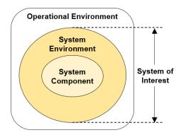
Figure 4. The structure of a system of interest in SAE
