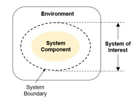
Figure 3. The system boundary of a system of interest
