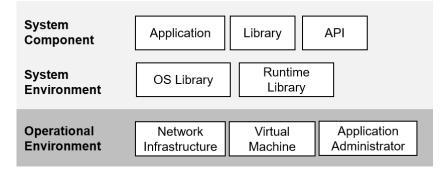
Figure 5. The structural composition of an application-software system
