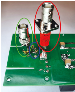
(D) Bottom from the side without DUTs. Left to right: Coaxial Gate-Source voltage probing point (green), Drain-Source voltage probing point (PCB pin receptacles, blue), coaxial CVR (red).
