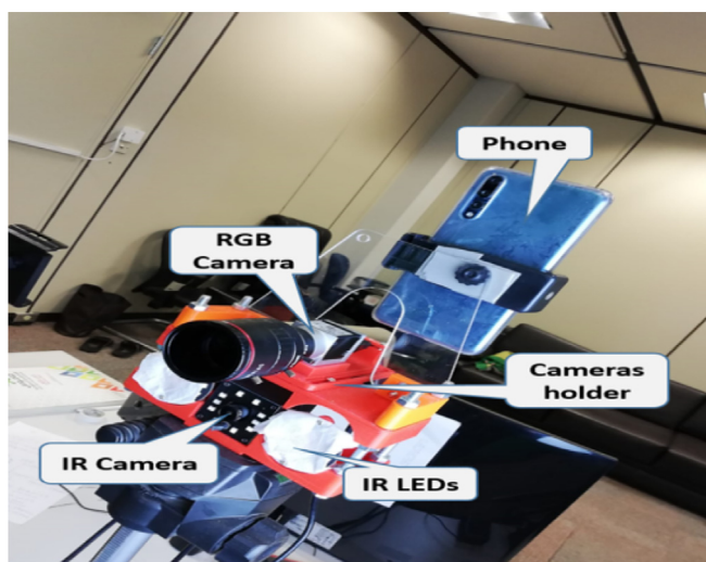
Fig. 4. Support for the cameras and the phone.
