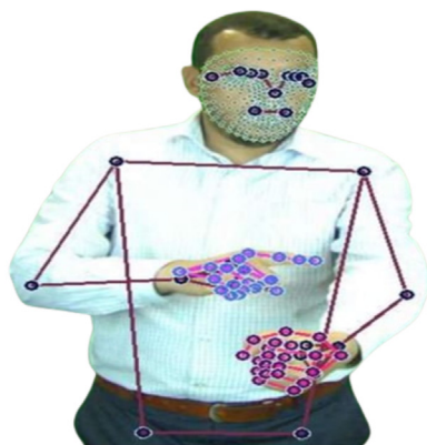
Fig. 11. MediaPipe landmarks (sample from our proposed dataset).
