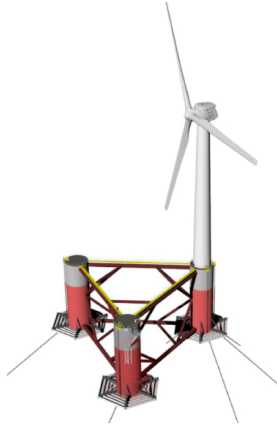
Figure 2.10: WindFloat - Principle Power, displaying heave plates on a semi-sub concept.
