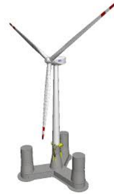
Figure 2.11: OO-Star - Dr. Techn. Olav Olsen, concrete semi-sub concept.
