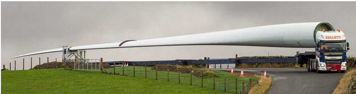
Figure 2.6: Transportation by truck of 58.7 m blades.
