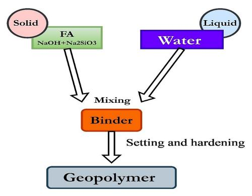
Figure 4. Dry mixing geo polymerization.
