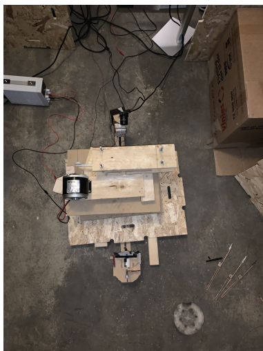
(a) Topside view of the camera rig with the lens moving mechanism placed between the LED_{12} and the bird model.
