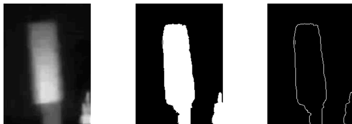
Figure 5.28.: Motion blur for the video-configuration FPS:20, shutter:1/20s, gain:16. Left: Grayscale image cropped out of the original frame. Middle: Otsu thresholded version of the left image. Right: Edge of the thresholded image, obtained with Canny edge detection.
