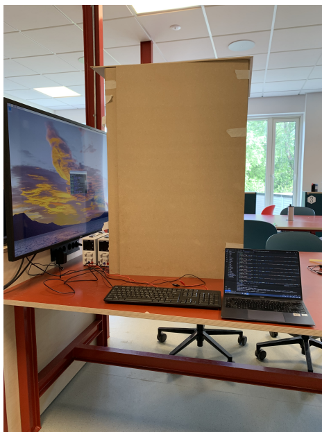
Figure 5.2.: Box isolated with MDF plates in the test location.
