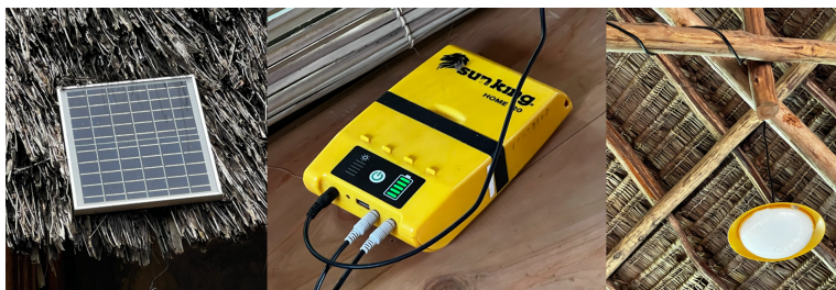
Figure 9: An example of a small SHS at Eco Moyo Education Center in Kenya [21].
