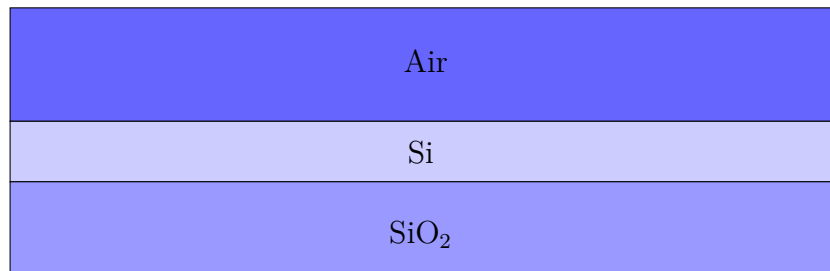
Figure 3.4: Effective mode index setup. The model is a 10\ \mu\text{m} long structure, with a 1\ \mu\text{m} thick \text{SiO}_2 layer on the bottom layer and a 220\ \text{nm} thick waveguide of Si on the top layer. The air layer is 2\ \mu\text{m} thick.
