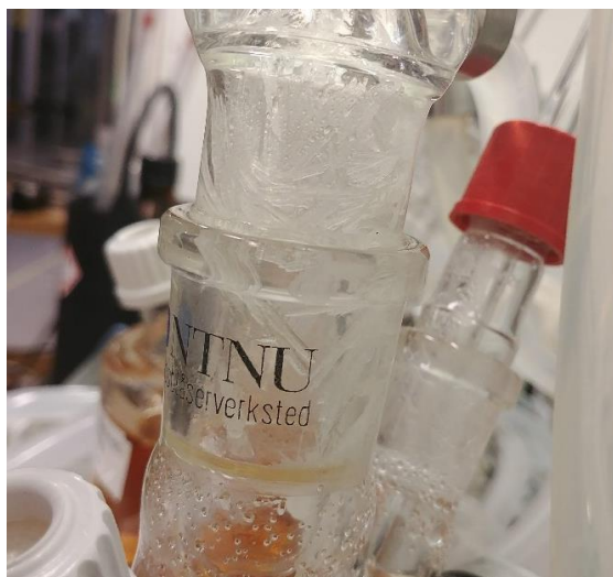
Figure 6.1.1: Crystalline structures formed in the connection between the reactor and cooler during the experiments with 5 Molal MEA in 80wt% TEG.
