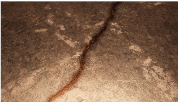
Figure 3.32.: Rendered image of a crack with a Crack Width of \simeq 1mm .
