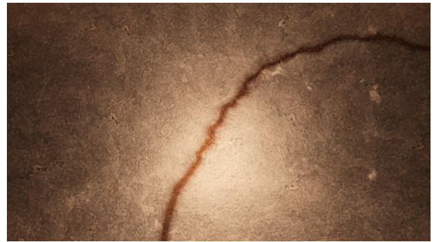
Figure 3.15.: Rendered image of a crack with a Noise Texture W of 40.
