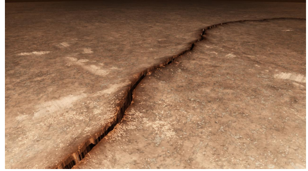
Figure 3.43.: Rendered image of a crack with a Crack Edge Height of 100\text{mm} .
