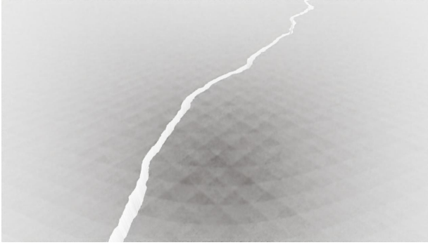
Figure 3.57.: Rendered wireframe of the subdivided crack plane. Here we can see the subdivided mesh with its edges and vertices. It is impossible to see the individual subdivided polygons as the final size of a polygon has become approximately half a pixel.
