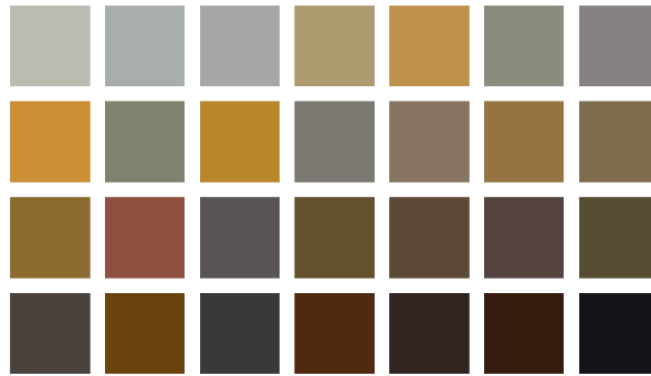
Figure 4.19.: RGB triplets gathered from DNV crack images using K-Means clustering. These RGB triplets were captured to have representative colours found in ship tanks during surveys. These are used to colour the PBR and procedural textures.
