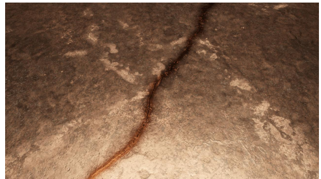
Figure 3.33.: Rendered image of a crack with a Crack Width of \simeq 2mm .
