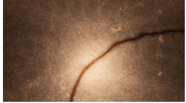
Figure 3.19.: Rendered image of a crack with a Noise Texture Scale of 2.75.
