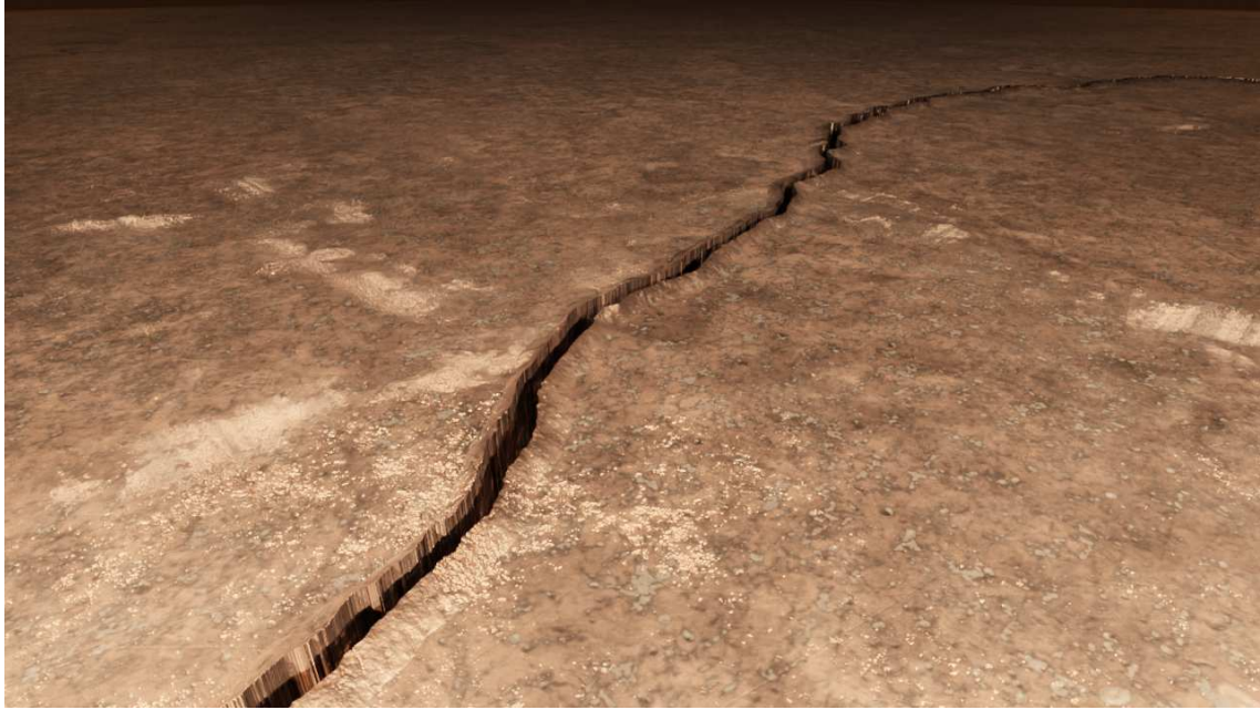
Figure 3.48.: Rendered image of a crack with a Crack Edge Height of 100\text{mm} , and a Corrosion Spread of 750 .
