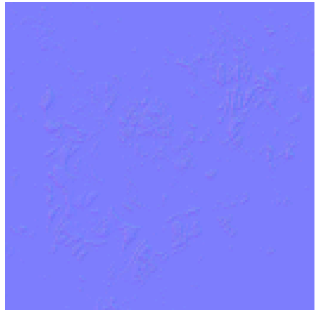
Figure 4.7.: Zoomed in normal map from figure 4.6 for the PBR material shown in figure 4.10. Here the variation in colours that are used to represent X, Y, and Z coordinates of the surface normal at that point is observed.
