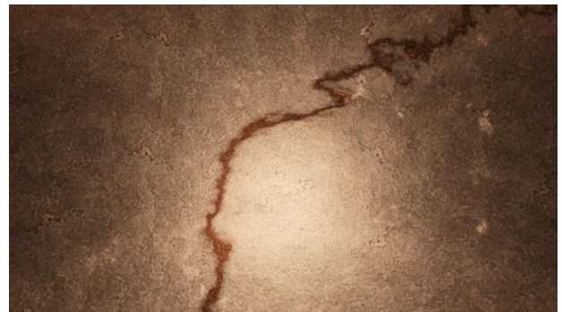
Figure 3.11.: Rendered image of a crack with a Noise Mix of 0.6. Here we observe that the noise added to the crack is too large, causing an unwanted crack representation.
