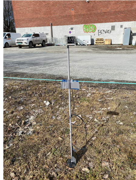
(b) Transmitter using external power bank as power-source.
