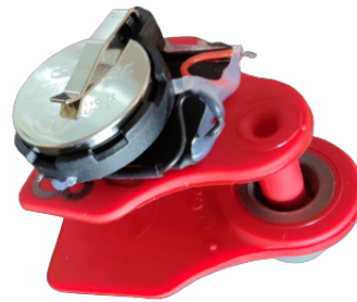
(b) Ear tag prototype using the Minew module. Picture from [6].
