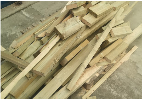
Pressure treated timber cut-offs
