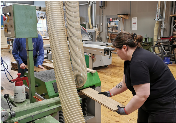
FIGURE 94. Planing oak flooring boards in NTNU wood-shop
