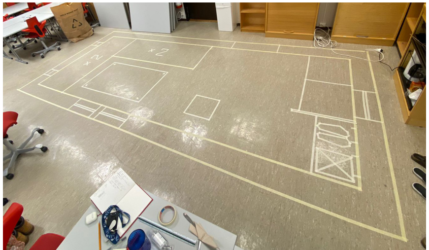
FIGURE 24. SPACE FOR INTERIOR IS TAPED TO THE FLOOR (PRIVATE PHOTO)
