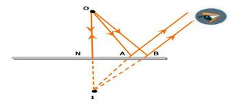
Figure 2. Construction of a virtual image using a ray diagram (TB8, p. 147).
