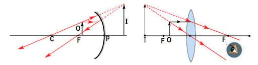
Figure 8. Representation of virtual image formation by a lens and spherical mirror (TB8, pp. 153 and 163).
