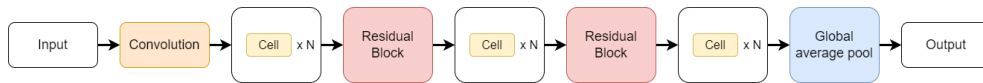
Figure 2.9: Depiction of the fixed macro architecture specific to NAS-Bench-201. The quantity of cells, denoted by N , along with the characteristics of the cells themselves, are variables subject to change
