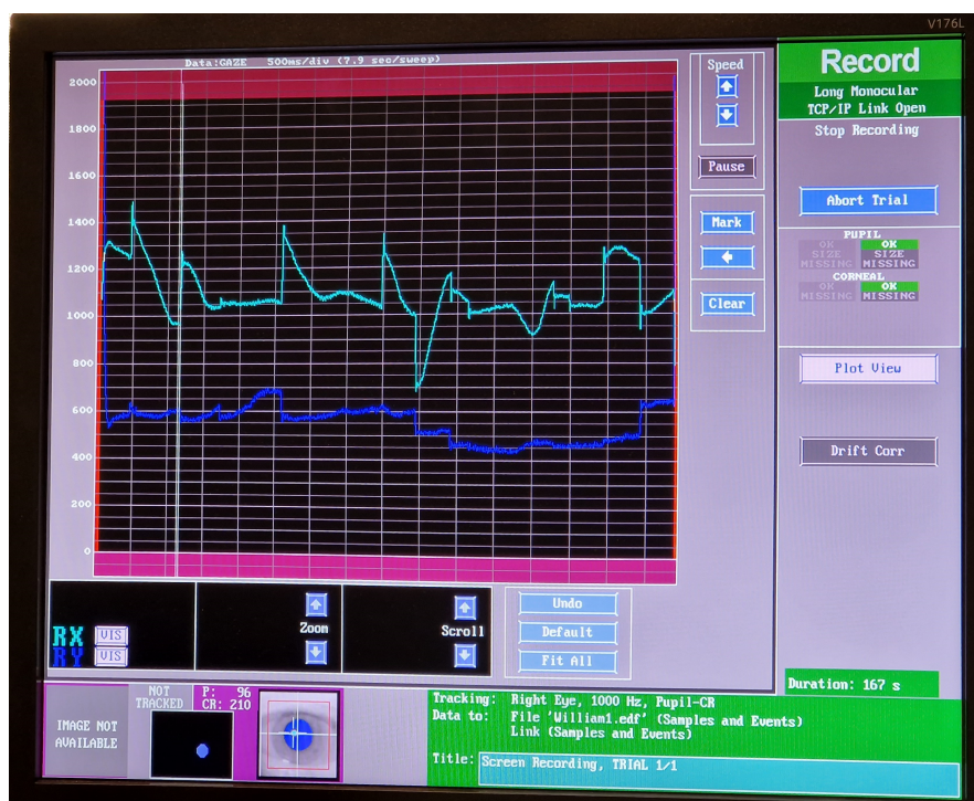
Figure H.0.2: EyeLink monitor observations with excellent calibrations
