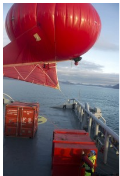
Helium balloon fitted with a specialized video camera.
