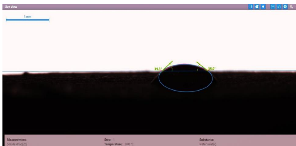
Figure 7. Contact angle for a disc of a core sample soaked in crude oil and PSC HMF (0.63 wt.%) at 60 °C.
