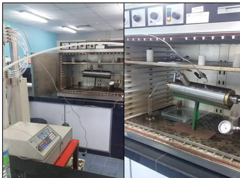
Figure 39. Main core-flooding apparatus used in experimental work.
