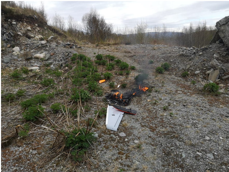
Figure 4.4: The burning Skywalker X8 UAV post-flight, with the 3D-printed ice shapes attached to the leading edge of the wing.
