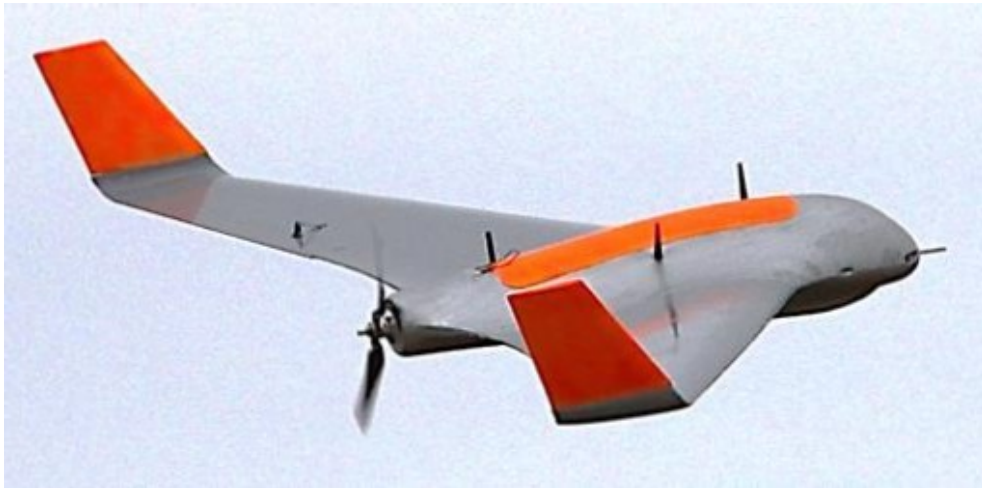
Figure 1.1: Skywalker X8 flying wing UAV. Source: NTNU UAV-Lab
