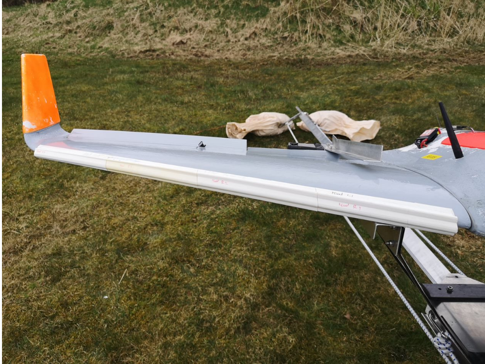
Figure 3.2: Right wing of the Skywalker X8 at Breivika equipped with 3D printed ice models. The image is taken pre-flight during safety checks.
