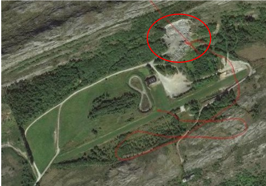
Figure 4.3: The image shows the final telemetry log updates from the Skywalker X8 in the gravel pit by the ground station. The red circle shows the crash site where it was found burning.
