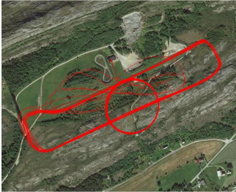
Figure 4.1: The racetrack pattern for the system identification experiments. Reconstructed by Ardupilot estimates during flight experiments. Maneuvers were performed on the long sides of the rectangle.
